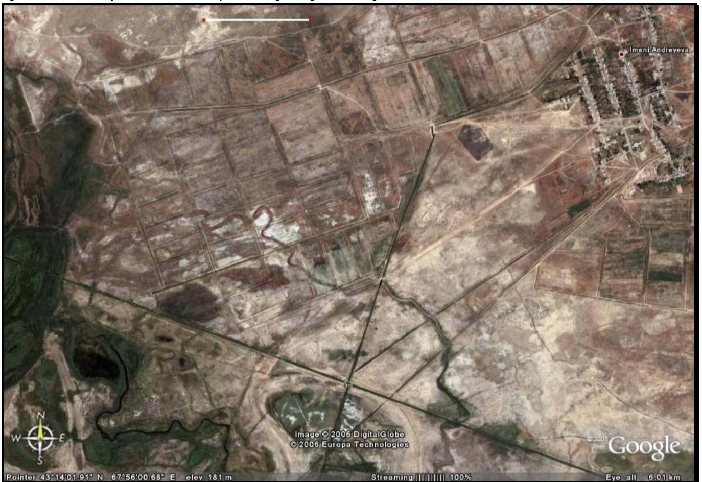
Figure H.18. Soil salinity accumulation due to poor drainage design and management, SW of Turkestan.
