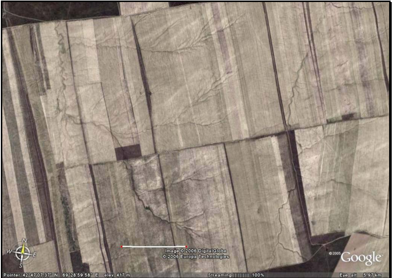
Figure H.12. Erosion rills and incipient gullies caused by cultivation in slopewise-direction (scale bar 1km)
